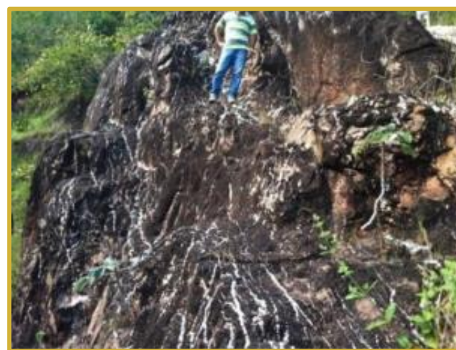
TYPICAL QZ VEINLETS WITHIN ORE ZONES
